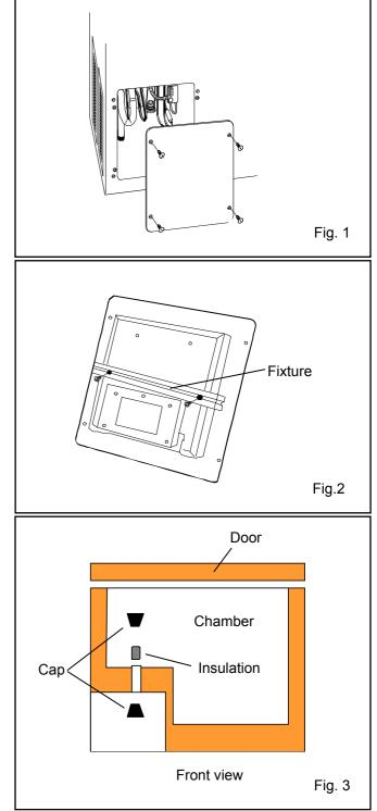
**4.** Remove the caps and insulation covering the access port on the chamber side and unit compartment side. (Fig. 3)
